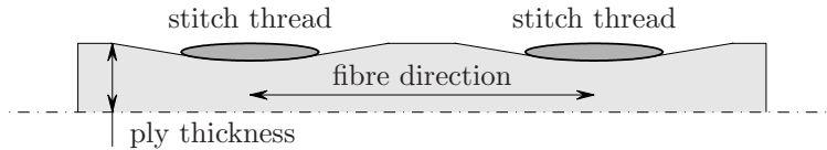
Figure 2.32: Cross-section of the fibre bundles (light gray area) in longitudinal direction. The dark gray areas represent the cross-section in transverse direction of the stitch threads which are pressed into the fibre bundle.
