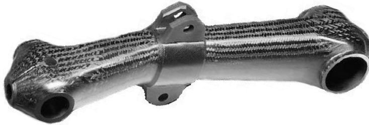
Figure 1.2: Composite trailing arm of the NH90 helicopter. (Braided at Eurocarbon, RTM-injection done at NLR).
